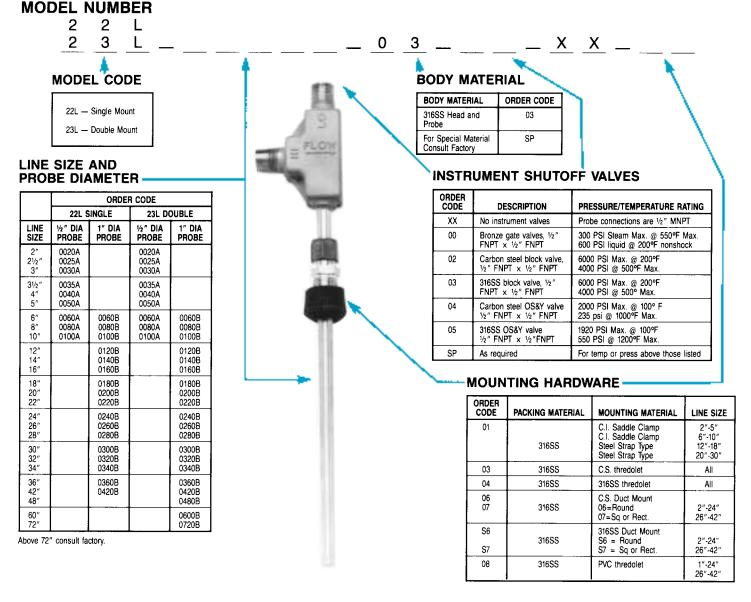
**SERIES 22L—ACCUTUBE—SINGLE MOUNT.** The Accutube Series 22L Probe is constructed of 316LSS cast head and 316LSS probe. The Series 22L probe has single-mounted support and installs through a single packing gland and thredolet. The Series 22L Accutube is factory-fitted with 1/2" NPT connections and is shipped with mounting hardware complete. Series 22L Accutubes are available for line sizes 2" through 42".
