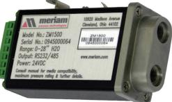
Meriam's compact, M1500 Analog or Digital Pressure Transmitters are ideal for pressure measurement needs from 10"  $H_20$  to 3000 PSI Full Scale. Output options include digital (RS-232, RS-485 and USB) or analog (mA or V DC). Choose from differential (dry/ dry or wet/wet), gauge, compound or absolute pressure types – see the table below for complete details.
