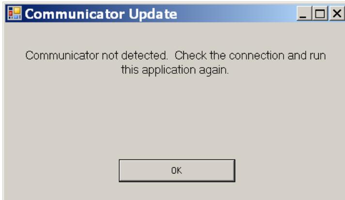
**This indicates there is an error with the hardware connection, or the drivers. Confirm there is power to the charger/communication base and it is connected to the PC. Confirm the field communicator appears in the Windows Device Manager under Ports (COM & LPT). The name of the device in the Device Manager is "Field Communicator". Then try the application again.**
