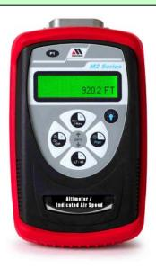
The Meriam Process Technologies (Meriam) M203 Altimeter / Indicated Air Speed Tester is a microprocessor based pressure sensing device used to measure pressure 0-900 millimeters (mm) Hg relative to absolute zero. The handheld is NIST traceable.
