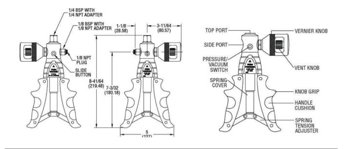
The M-600KT Combo Pneumatic Calibration Hand Pump comfortably sources pressure and vacuum to check calibration of gauges, switches, transmitters and recorders. The contoured cushion handles provide extra comfort while preventing the pump from sliding. The oversized check valve provides smooth operation throughout the output range. The dual o-rings on all pistons insure zero leakage.
