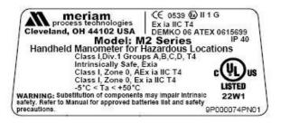
Intrinsically Safe versions are shipped with Dwg. No. 9R000056 "M2 Series Intrinsically Safe Control Document". Refer to this document for details of the certification, a list of warnings and a list of approved batteries for use in Intrinsically Safe versions.
