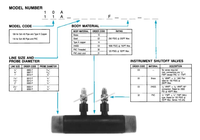
**SERIES 10A** inline sensors are supplied in threaded Schedule 40 pipe nipples (except for the type "K" Copper). The inline sensor is complete with factoryfitted probes and is supplied as a complete assembly providing for economical installation. Series 10A sensors are supplied with Steel, 316SS, Brass, and Type "K" copper. Available in line sizes ½" through 3".
