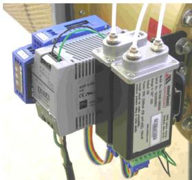
DIN rail mounting is accomplished using the factory-installed DIN clip located on the edge of the M1500 enclosure. DIN rail mounting is excellent for mounting several M1500s in close proximity to one another, either inside a protective enclosure, or on a convenient mounting surface or wall. For high vibration applications use the longer panel mount screw to secure enclosure to DIN rail.
