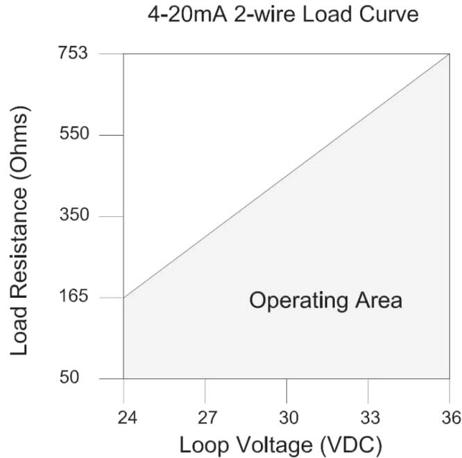
Max Load Resistance = 753 Ohms (at 36 VDC)
