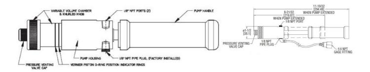
The MP-100KT Calibration Pump features a Delrin® plastic handle that prevents body heat transfer from interfering with readings, as well as an oversized check valve for smooth operation. The dual o-rings on all pistons insure zero leakage.
