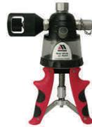
**MH-600KT Hydraulic Calibration Pump** uses a fully adjustable stroke control to allow for fast priming or filling of test systems. This gives the operator the ability to switch as needed to a smaller stroke for easier pumping at high pressure. Each MH-600KT includes a black padded canvas case and a 2ft non-stretch hose and fittings. It is backed-up with a 2 year warranty.
