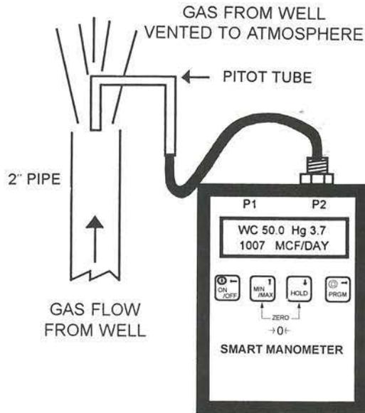
and eliminates the need to use an AGS table for conversions. The open flow manometer displays the flow rate from the well in thousands of cubic feet per day, and it also displays the differential pressure in the appropriate units.
