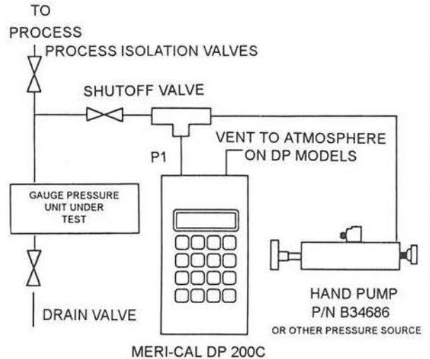
digital manometer. Compared to other calibration techniques, a digital manometer calibration is fast and simple. There are no cumbersome boxes, gas cylinders, regulators or weights to set up; and no special platforms or critical procedures for leveling.
