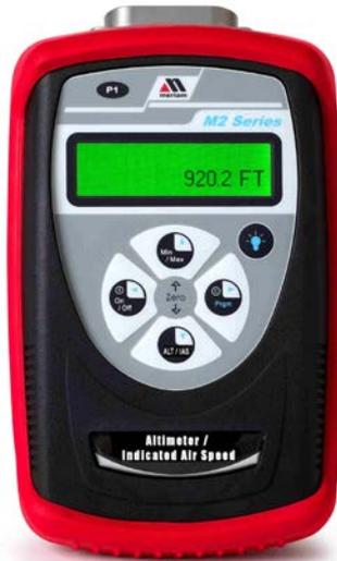
The Meriam Process Technologies (Meriam) M203 Altimeter / Indicated Air Speed Tester is a microprocessor based pressure sensing device used to measure pressure 0-900 millimeters (mm) Hg relative to absolute zero. The handheld is NIST traceable.
