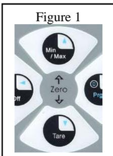
NOTE: The M203 can be zeroed only if the new applied zero is within ~ 1% FS of the original factory calibration zero. If outside this limit a "ZERO RANGE ERROR" message appears and the manometer will not zero. Contact the factory for support in this case.
