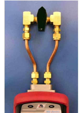
QTV Manifold ¼ Turn Valve is manually opened to equalize DP sensor and closed to make readings
