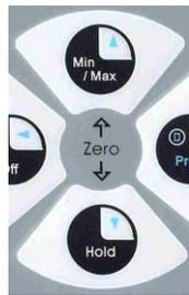
**Note:** *The smart manometer can only be zeroed if the new zero value is within  $\pm 5\%$  (of FS) of the original factory calibrated zero. If the zero procedure generates a new zero value outside this limit, a ZERO RANGE ERROR message appears indicating that the procedure failed. Factory service may be required.*
