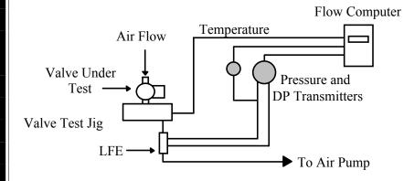
This depicts vacuum testing a valve. Testing a valve for a pressurized flow is done by simply reversing the flow direction. Standard LFEs are calibrated for flow in one direction only. If a test stand is to be used for both vacuum and pressure testing a bi-directional calibration should be requested.
