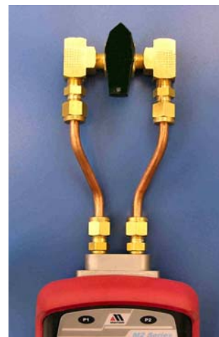
QTV Manifold ¼ Turn Valve is manually opened to equalize DP sensor and closed to make readings
