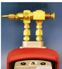
PTR Manifold Valve is open and DPVa sensor equalized until the push button valve is
